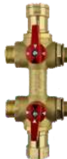
Valve shown in normal operation mode with water flow and return through the water softener and installed on vertical pipe.
